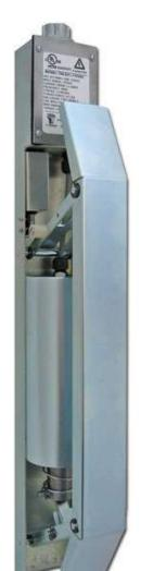
The C.J. Anderson Retiring Cam (ARC), made in the USA, is a Self Contained Retractable Cam. Its modular design permits replacement of all component parts in the field. This is a 2.75" wide by 12.25" long cam which can be used on any type of door lock.
