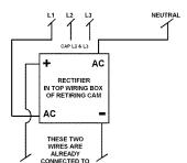
When replacing a 3 Phase Motorized Cam, simply connect one "HOT" phase to the AC Side on the rectifier and the other AC to a common or neutral if you are replacing a 220. To ensure that your retiring cam lasts as long as possible connect as shown! If you connect to of your "HOT" lines to the cam this will create the unit to heat up prematurely and decreases the life of the cam.
