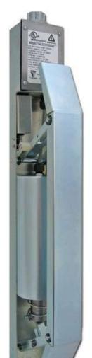
The C.J. Anderson Retiring Cam (ARC), made in the USA, is a Self Contained Retractable Cam. Its modular design permits replacement of all component parts in the field. This is a 2.75" wide by 12.25" long cam which can be used on any type of door lock.
